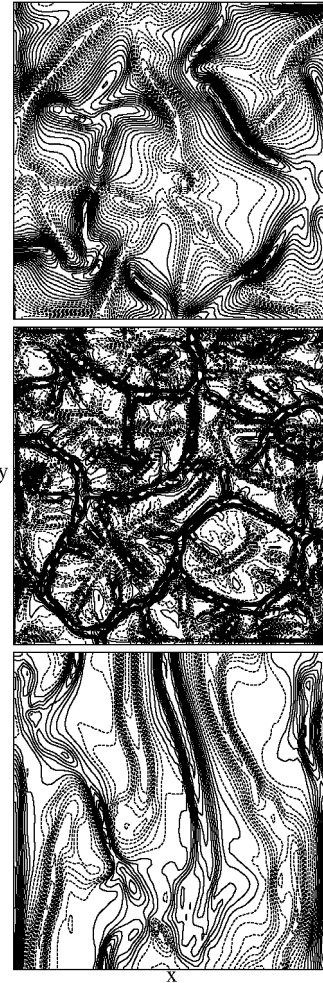
Fig. 8. Vertical velocity \langle W \rangle distribution in the central horizontal (x-y) plane ( z/D = 0.5 ), Ra = 10^7 , Pr = 0.025 . Above: Ha = 0 , no magnetic field, \langle W \rangle_{\min}^{\max} = \pm 0.4 ; middle: Ha = 200 , transversal magnetic field ( \mathbf{B} \parallel z ), \langle W \rangle_{\min}^{\max} = \pm 0.45 ; below: Ha = 200 , longitudinal magnetic field ( \mathbf{B} \parallel y ), \langle W \rangle_{\min}^{\max} = \pm 0.55 .
